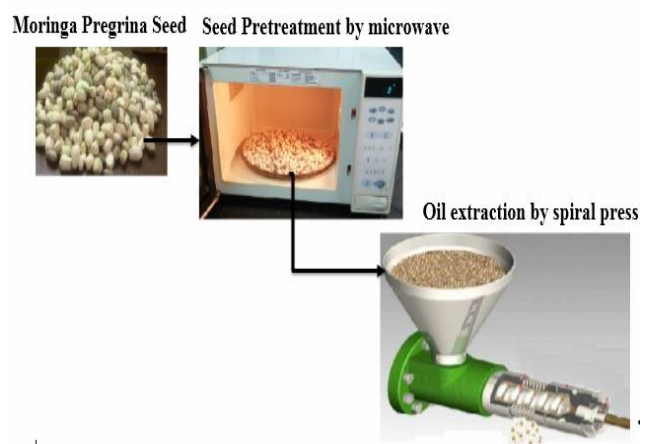
Fig 2 Schematic of mechanical extraction of oil from Moringa seeds.
