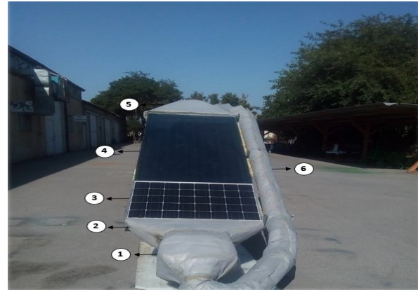
Fig 1 The combined photovoltaic / thermal solar dryer containing PCM
