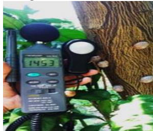
Fig 3 Measurement of light intensity with a lux meter device (Ghaemshahr- 2020)
