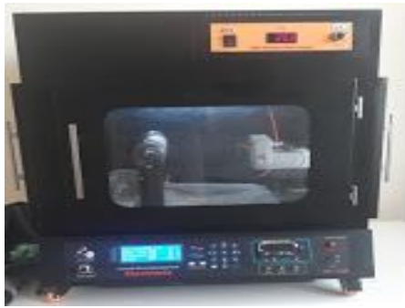
Fig 1 Electrospinning device used in this study
