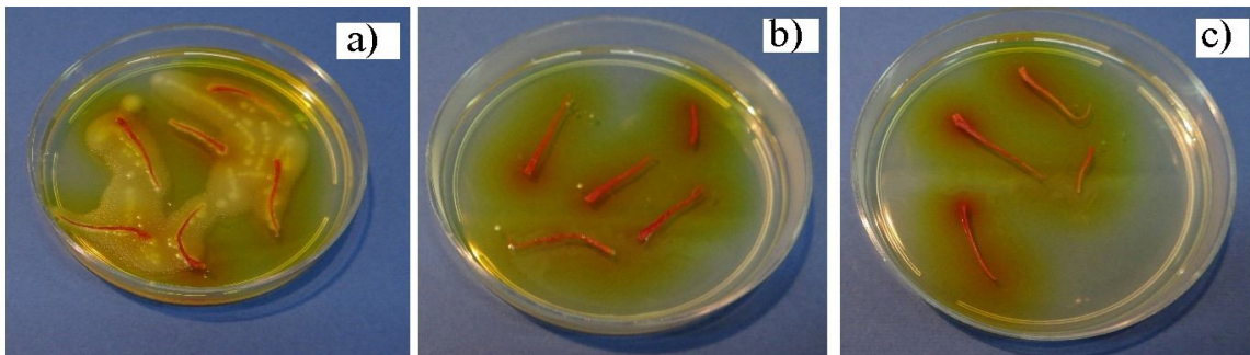
Fig 5 Bacterial disinfection effects of dielectric barrier discharge plasma in surface mode for a) control and b) 5 min c) 15 min plasma treated sample
