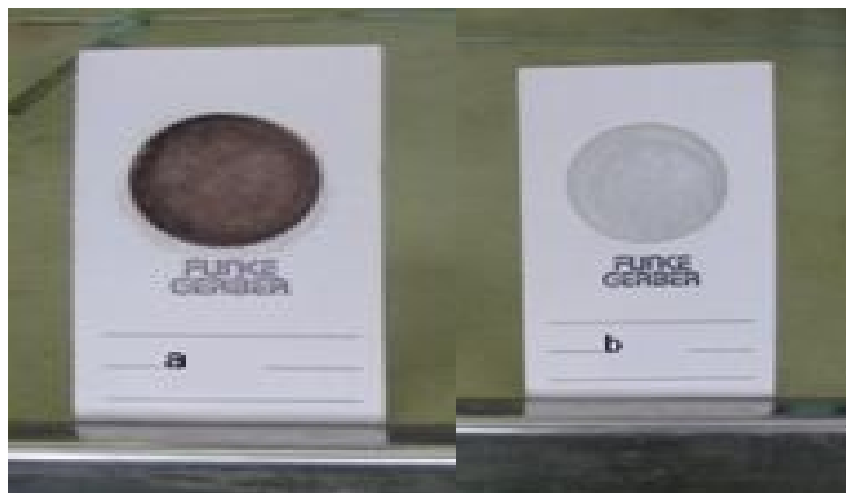
Fig 4 Scorched particles of low lactose cocoa milk powder (a) and low lactose banana milk powder (b)
