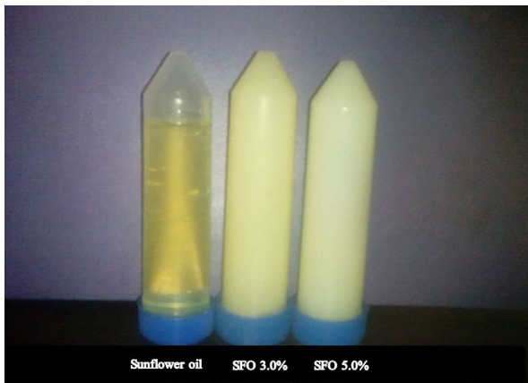
Fig 3 visual appearances of sunflower oil and structured sunflower oil (SFO) with 3.0 and 5.0% monoacylglycerols
