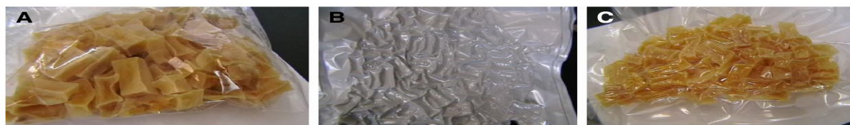
Fig 2 (A) Transpirant biaxially oriented polypropylene (BOPP) laminated; (B) polyethylene-polyamide laminate; (C) semi-transparent BOPP
