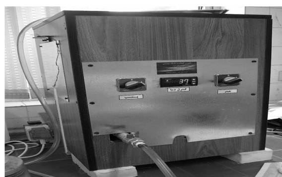
Fig D Water bath circulation
